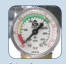
1 touch incorporates an Active Gauge that allows pressure reading, when the cylinder shut-off valve is closed. This will allow quick reading of the remaining quantity of gas contained in the cylinder. Special fluorescent dial provides great reading visibility in the dark
